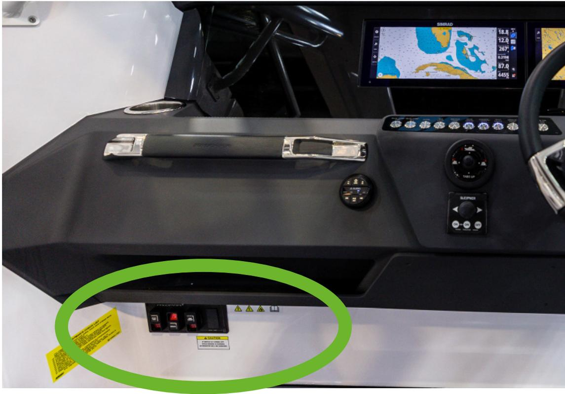
Remote controlled main switches, twin engine
