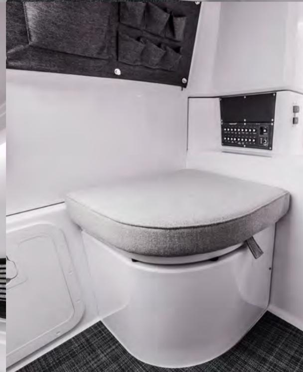
*You can opt for a cleverly hidden day heads with a 32L septic tank in the front cabin that can be easily accessed by lifting the cabin bench lid.*
